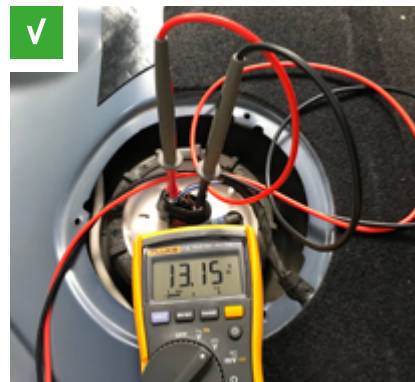
Fig. 2: Electrical plug contact on the cover of the fuel delivery module
