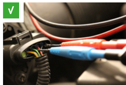
Fig. 3: Measuring tips on the rear of the plug
